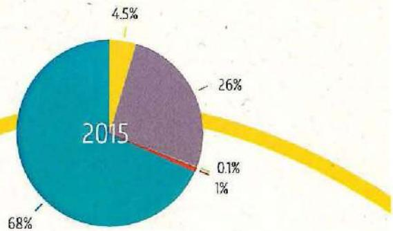
▲ The consumed electricity consists of ● purchased green energy (68%), ■ electricity produced by CHP units (4.5%), ▨ electricity generated by three wind turbines (26%) and ▲ solar panels (0.1%). The origin of the other energy is unknown ■; this is used in the rented buildings.
