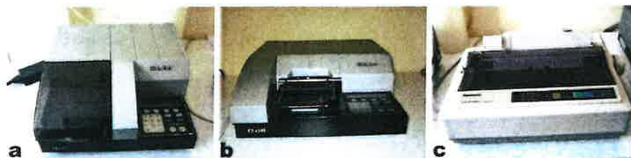
Fig. 4. Washer (a), reader (b) and printer (c) used in ELISA procedures.
